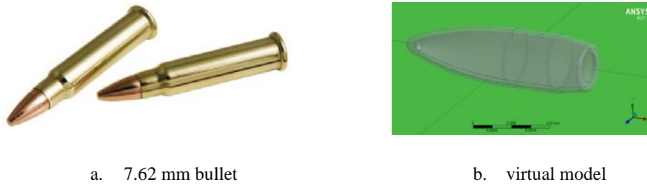
Fig. 5. Geometrical and computational model of the bullet
