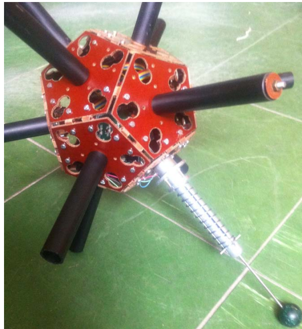
Fig. 8. The prototype leg integrated in the dodecahedron structure used for testing.
