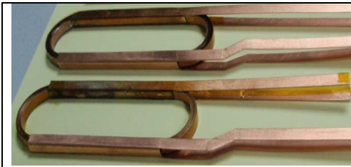
Fig. 1. HTS pancake coils for electric generator
