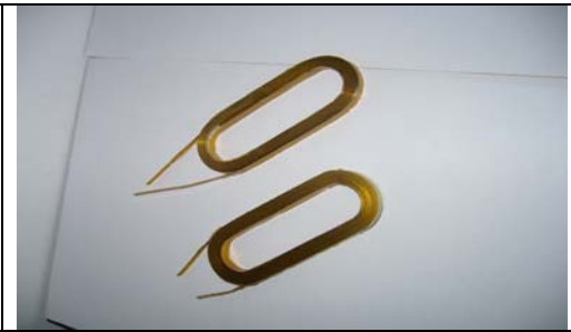
Fig. 2. Double pancake coils for synchronous electric motor
