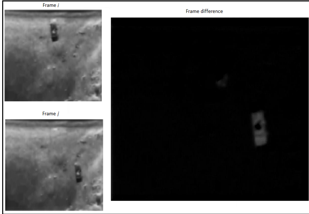
Fig. 1. Temporal differencing for two sonar frames
