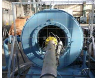
Fig. 4. Measurements for acoustic intensity to perform the compressor case mapping (49 grids surfaces \sim 18 \times 18 \text{ cm} each with a distance between them and case of 18 cm)
