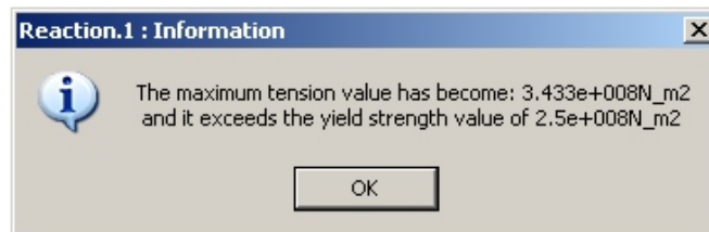
Fig. 10. The program calculates the maximum stress and compares it with the yield strength
