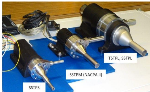
Fig. 1. Family of pumps for MPFL systems developed by Realtechnologie AG (now Nanospace) [5]
