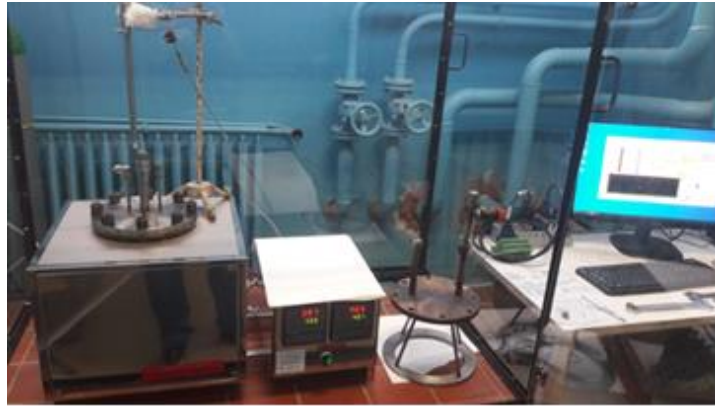
Fig. 2. Installation for corrosion tests in liquid lead
