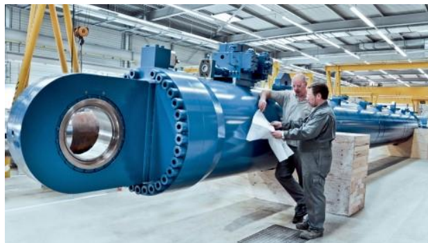
Fig. 13. Electrohydraulic servo cylinder for water gates ( Source: REXROTH ). [2]
