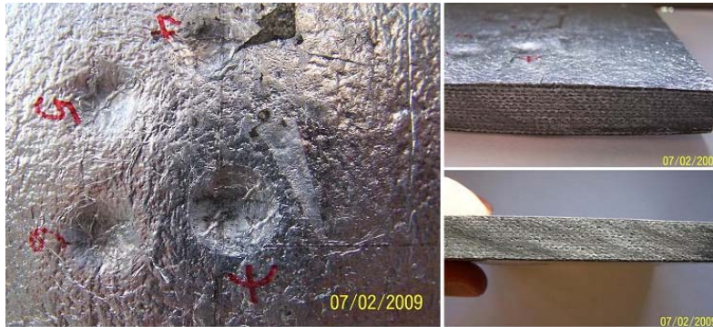
Fig. 12. Laboratory impact tests performed on a 14-layer CFRAI plate
