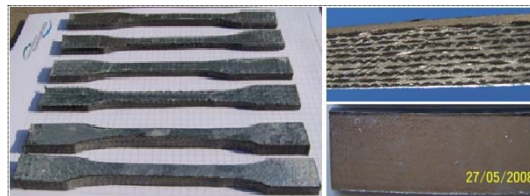
Fig. 6. CFRAI samples (tensile and ballistic test specimens)
