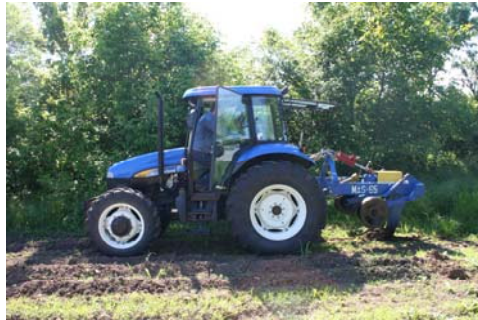
Fig.1. MAS65 deep soil loosening machine, aspects during experiments
