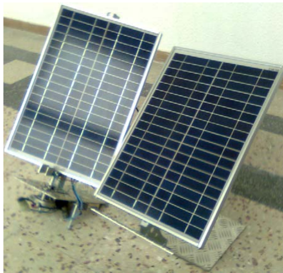
Fig. 2. Solar tracking PV panel and fixed PV panel used for comparison
