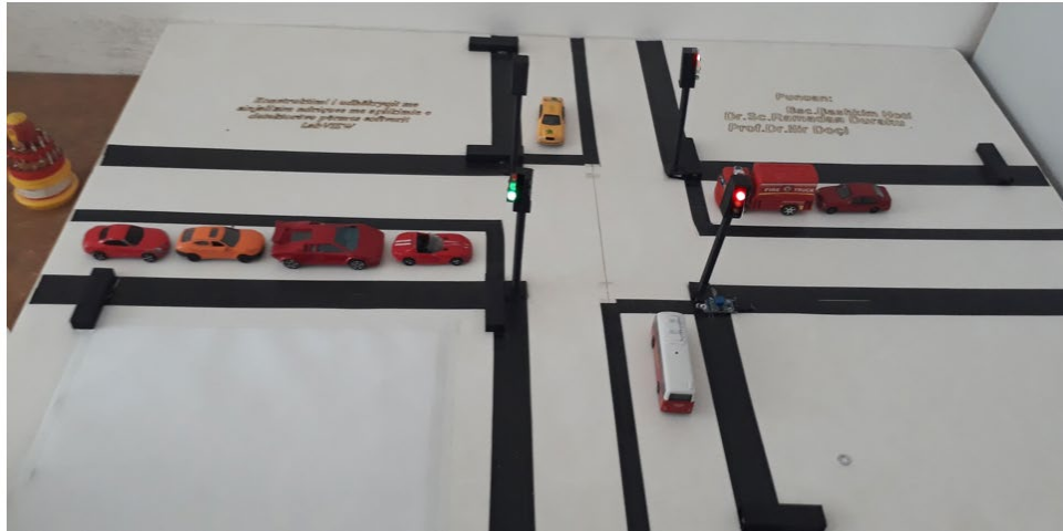
Fig.16. Case 4. EBT Lane has queues of vehicles (DPD Detector Activates). Receives priority with Green Color in the traffic Light.
