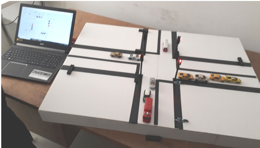
Fig.1. Model of Cross-type Intersection with Software Control
