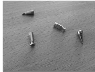
Fig.4. Analogues implants by DMLS
