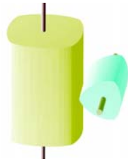
Fig. 15. Polycentric gear simulation i = +3/4 a
