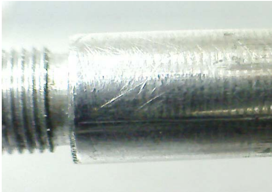
Fig. 13. Defects on the surface of the motor's shaft, caused by the manufacturing process and visible as transversal striations
