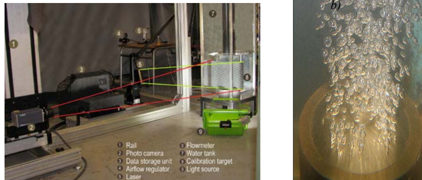
Fig. 1. a) Measurement set-up, b) Emissions of bubbles by perforated plates MP0.2.
