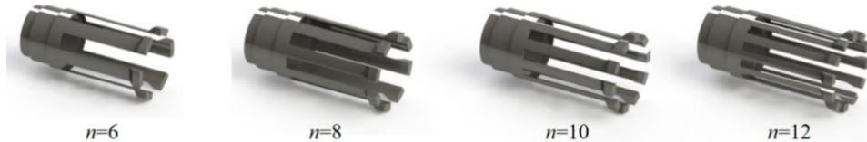
Fig. 12. The models of elastic claw with different number of claw pieces
