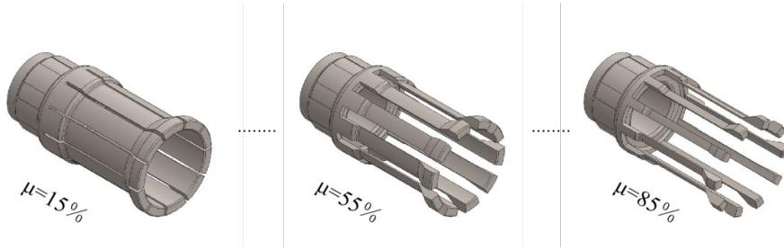
Fig. 13. The models of elastic claw with different claw width
