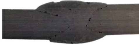
Fig. 10. Corrosion specimen after testing
