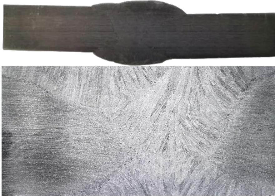
Fig. 6. Macroscopic examination specimen
