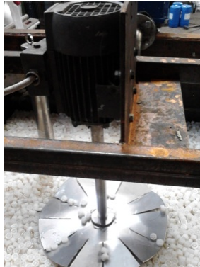
Fig. 3. Biofilm carriers inside the MBBR and a surface aerator/mixer
