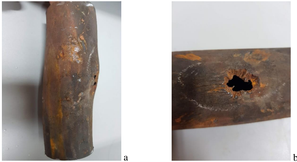
Fig. 4. Macroscopic image of damaged pipe 13 (a), detail of the sample right side (b)
