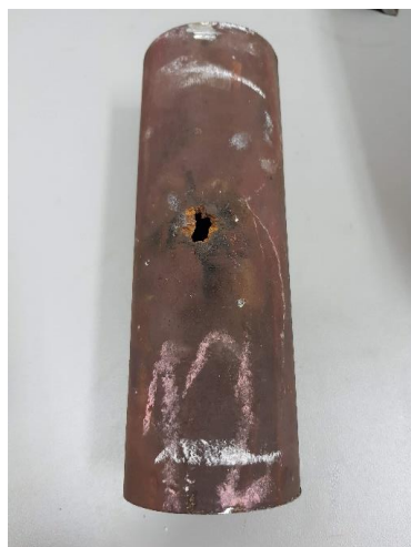
Fig. 3. Macroscopic image of damaged pipe 12 (a), detail of the sample front side (b)
