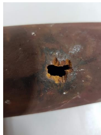
Fig. 3. Macroscopic image of damaged pipe 12 (a), detail of the sample front side (b)
