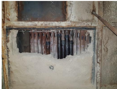
Fig. 1. Macroscopic overview of boiler pipes damaged in operation
