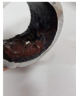
Fig. 2. Macroscopic image of damaged pipe 11 (a), detail of the sample inner surface (b)
