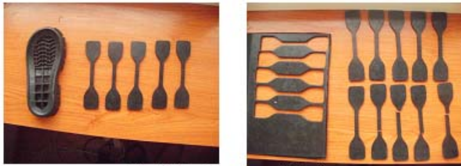
Fig. 2 CFP specimens prepared for testing
