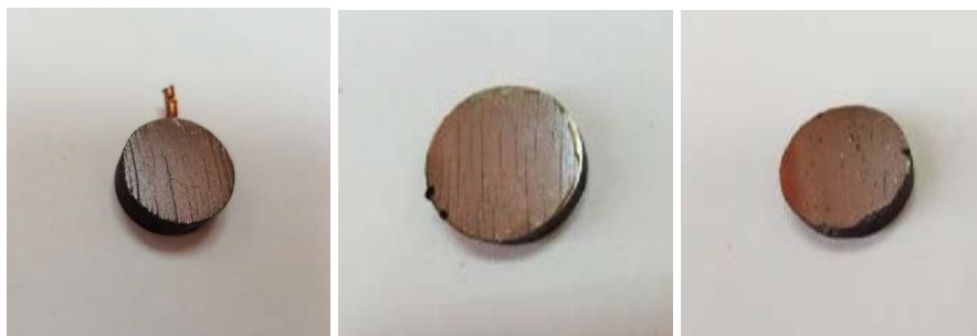
Fig. 9 Macro image of the three samples after the electrochemical corrosion test
