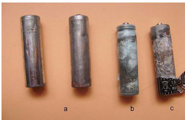
Fig. 7. Corrosion of a Zn-C battery AAA type: a) new batteries; b,c) spent batteries
