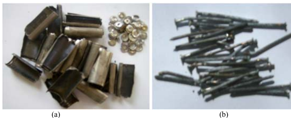
Fig.2. Metallic component: a) cathode current collector; b) anode current collector from bronze; ex. battery case, terminal ends, steel separators.
