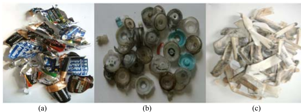
Fig. 3. Plastic, paper, cardboard: a) outer sleeves; b) support elements; c) separators in paper and cardboard insulators.
