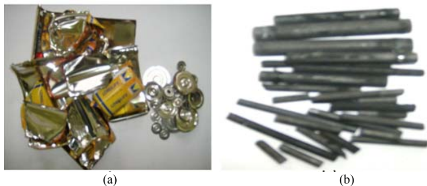
Fig. 5. a) Iron housing and terminal ends; b) cathode current collector from graphite.
