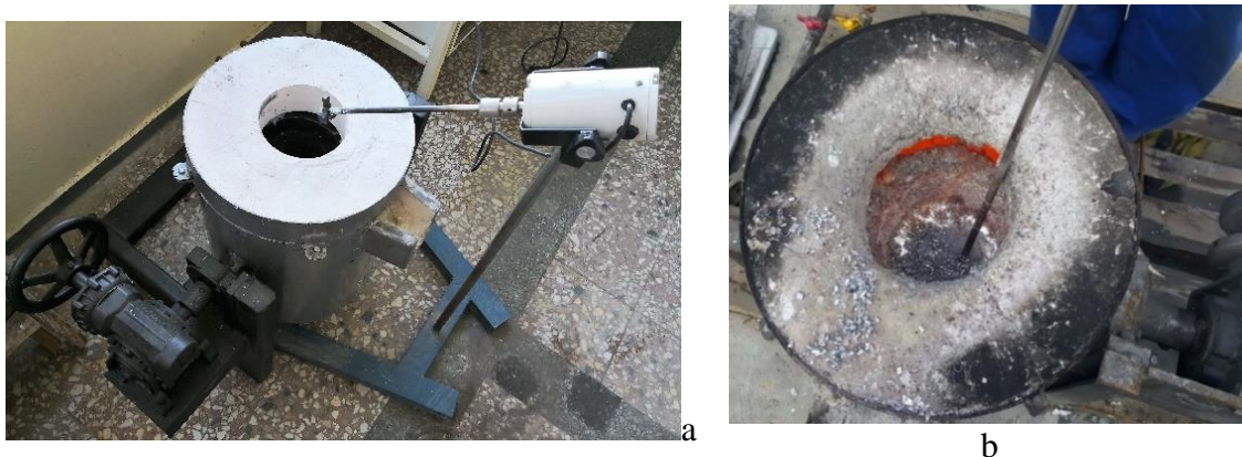
Fig. 1. The furnace used in the experiments for the semisolid/pasty melt with the agitator (a), the furnace filled with 10 kg of molten aluminium (b),
