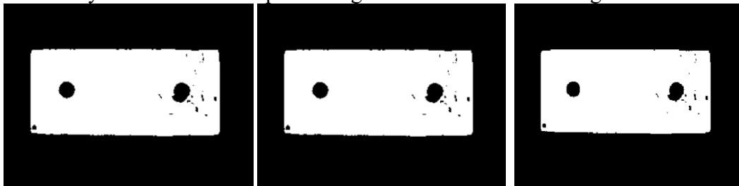
(a) Global fixed threshold method (b) Local adaptive threshold method (c) Otsu method
