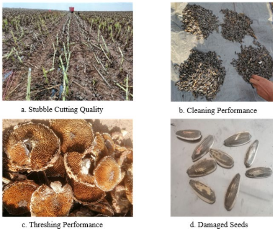
Fig. 13. Field Harvesting Performance of the Edible Sunflower Combine Harvester
