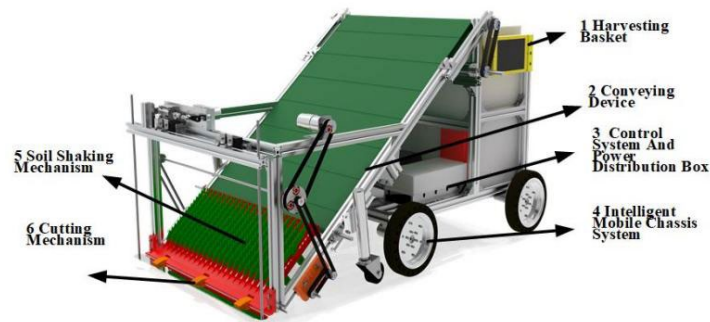
Fig. 1 The overall mechanism diagram of the Shaking soil spinach multifunctional automatic harvester
