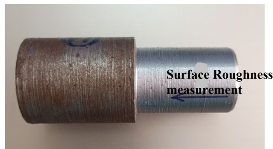
Fig. 6 Specimen showing direction of surface roughness measurement
