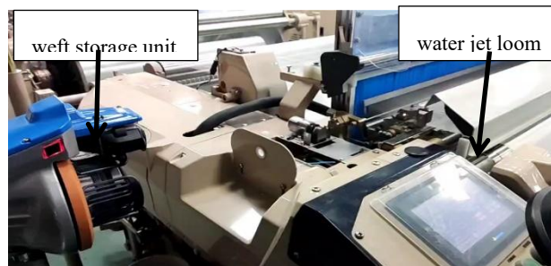
Fig. 6 Weft storage unit and water jet loom
