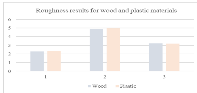
Fig. 8. Comparison of surface roughness values between wood-based composite and PLA
