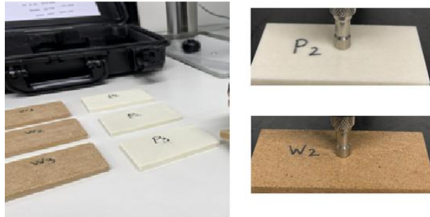
Fig. 3. Experimental setup for hardness measurements on PLA and wood-based samples
