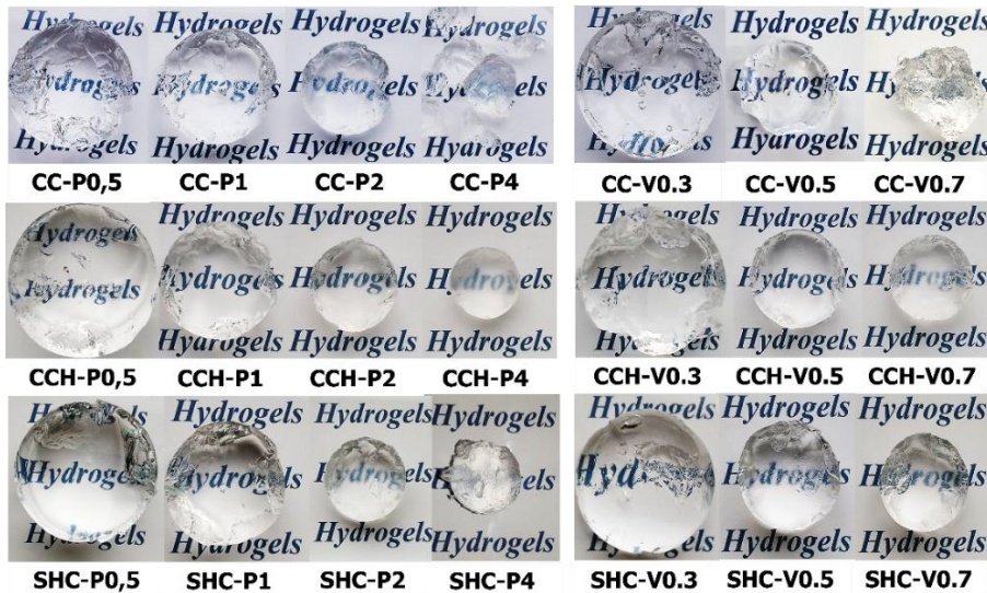
Fig. 1. Swollen hydrogels obtained from three types of chitosan and various monomer-to-crosslinker ratios, as expressed in Table 1.
