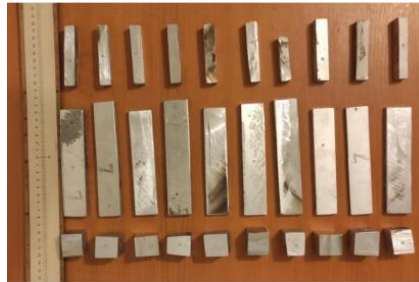
Fig. 1. Image of the macroscopic appearance of experimental specimens of alloy 2017A, with different dimensions for conducting experimental research
