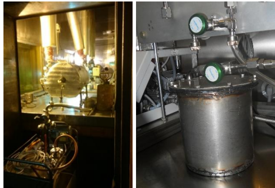
Fig. 4 Irradiation equipment - Gamma 5000 chamber containing a set of \text{Co}^{60} sources distributed circularly with an activity of 8000 Ci [18].
