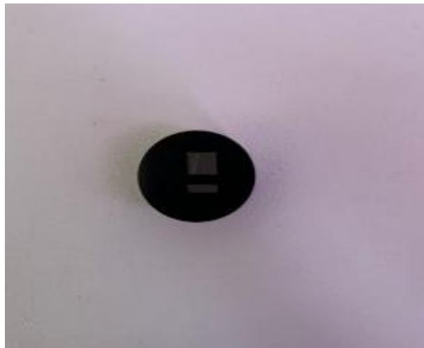
Fig. 4. Prepared metallographic sample
