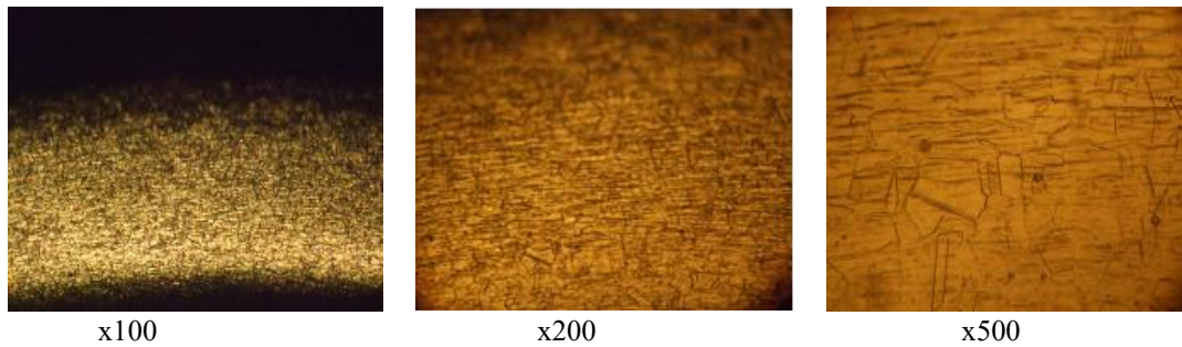
Figure 3. Material microstructure of cold-formed plate areas etched with Marble's reagent
