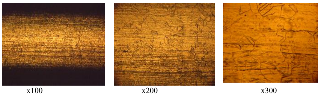
Figure 2. Microstructure of the material in the contour zones of the plates; etched with Marble's reagent
