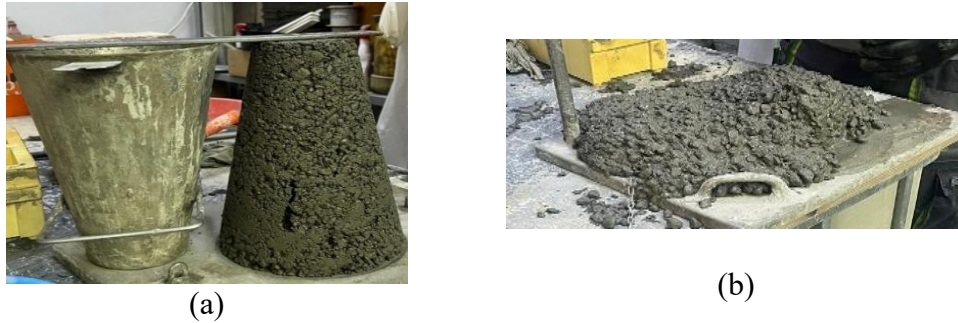
Figure 5. Concrete slump test: (a) C_RCA; (b) C_RCA-LA
