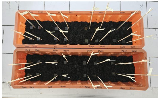
Figure 1. Experimental setup of the soil burial test after one week, showing the arrangement of the samples prior to soil coverage.
