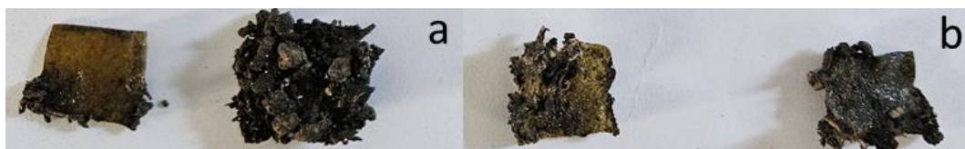
Figure 6. PVA80-MBH-SK-US (a) and PVA60-MBH-SK-US (b) samples after 1 week of soil burial.
