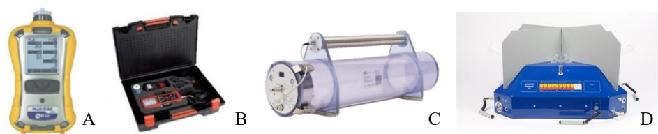
Figure 2. Multi RAE gas analyzer (A), Optima 7 gas analyzer (B), vacuum sampling system with nalophan sampling bags (C), Olfasense T08 dynamic olfactometer for 4 assessors (D).
