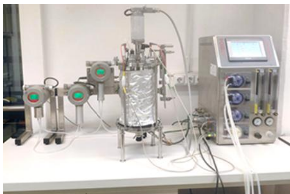
Figure 1. The EDF 5.4_1 bioreactor used in the AD process.
