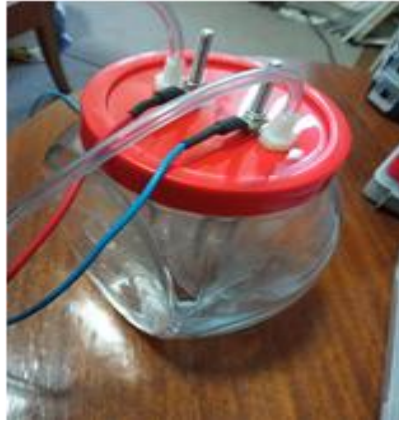
Fig. 3. The can used for gas capturing and filtering
