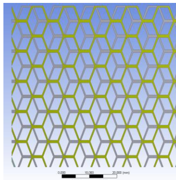
Fig. 5. Second geometrical configuration for the multilayered honeycomb composite material
