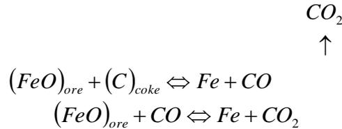
In order to make cast iron and steel, the direction of the above reactions must be permanently maintained to the right. This means that the production of ferrous materials is a process that generates CO<sub>2</sub> *objectively and mandatory*.
