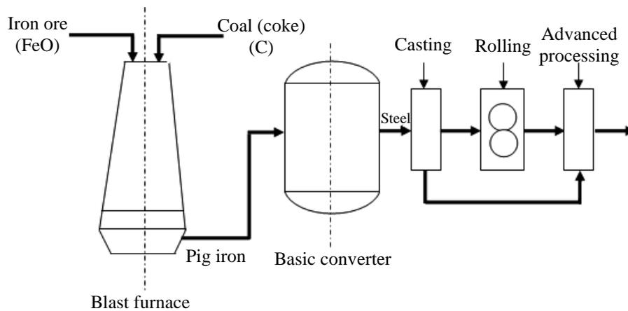
Fig.2. Technological flow (→) in iron and steel-making industry
