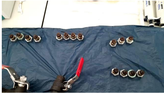
Fig. 3. The studs with disk coupons on which the biofilm accumulated
