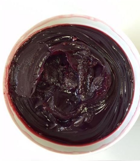
Fig. 3. Grease made experimentally from waste oils (experimental research 1)
