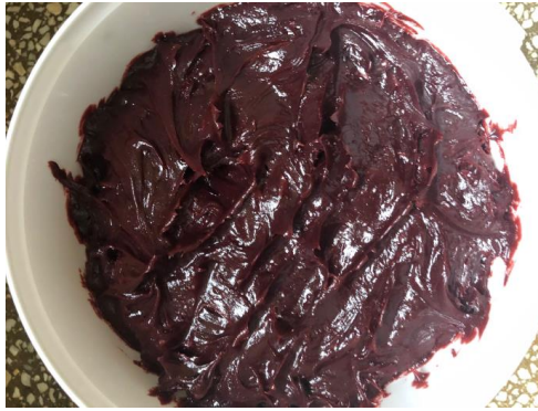
Fig. 4. Grease made experimentally from waste oils (experimental research 4)
