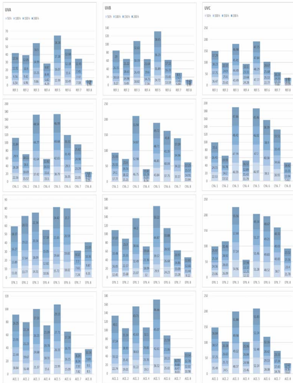
Fig. 2 – variation of the overall color difference ( \Delta E^* ) with exposure time and UV irradiation source on selected test blocks: REF – control samples, CYA – cyanoacrylate, EPX – epoxy resin and ACE – acetone infiltrant block samples; 1 to 8 color set: red, green, blue, yellow, magenta, cyan, uncolored, grey
