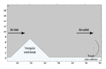
Fig. 1. The trough solar collector with windbreak of the present work.
