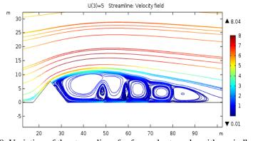
Fig. 8. Variation of the streamlines for four solar troughs with a windbreak.
