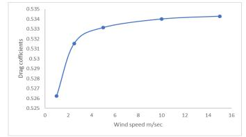
Fig. 6. Values of drag coefficients for four troughs without windbreak.
