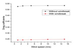
Fig. 10. Drag coefficients for four troughs, with and without windbreak.
