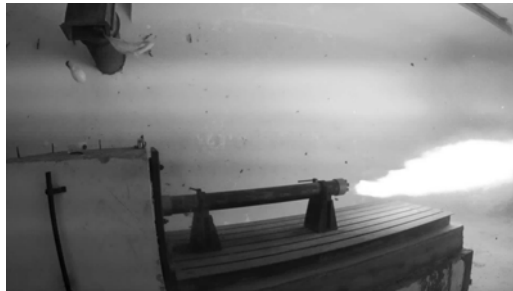
Fig. 5. Composite SRM during firing test. Fig.6. Double base SRM during test firing.
