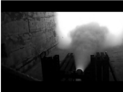
Fig. 5. Composite SRM during firing test. Fig.6. Double base SRM during test firing.
