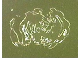
Fig.11 Site destroyed on a commercial dielectric mirror at 7 mJ energy, single-pulse.
