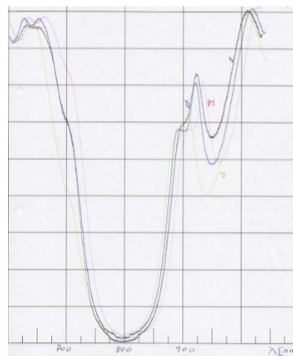
Fig.3 Transmissions of some witness plates at an incidence of 45 deg
