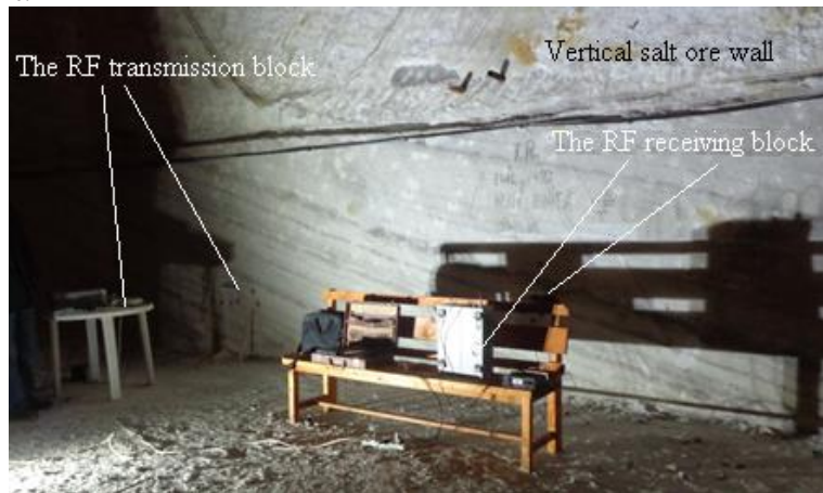
Fig. 8. The complex system of the determination of the dielectric parameters in saline environment for detecting the Cherenkov cone of electromagnetic radiation in this medium at the frequency of 187.5MHz with the two blocks (emission and reception).
